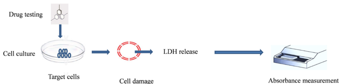
Fig. 1 – Principles of measuring cytotoxicity using the lactate dehydrogenase (LDH) test.
